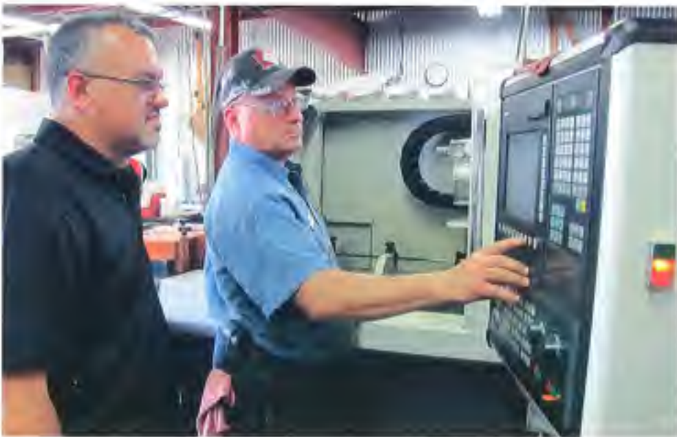
Shop owner Christian Klanica (left) and machinist Tim Wolf review programs for jobs scheduled to run on the deep-hole machine. The Siemens 828D control enables shopfloor programming of three-axis work, including automated routines for bolt-hole circles and other patterns.
